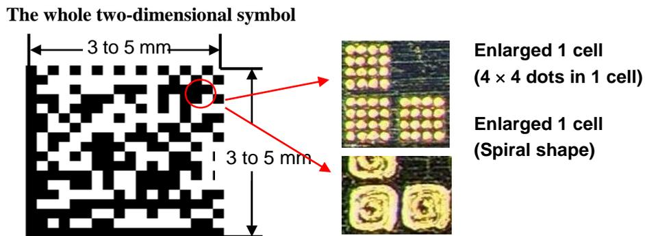
Figure 5. Example of Marking Pattern of Cell
