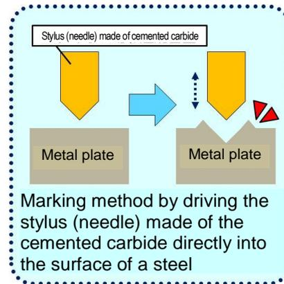
**Figure 3. Marking Mechanism of Dot Pin Method**
