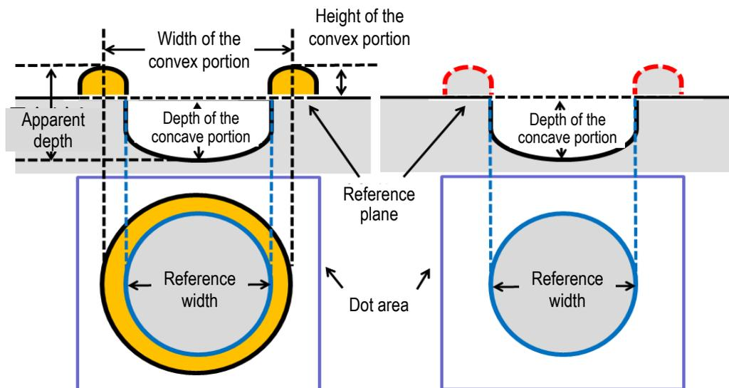
a) Dot shape with an instrument not used      b) Dot shape with an instrument worn
